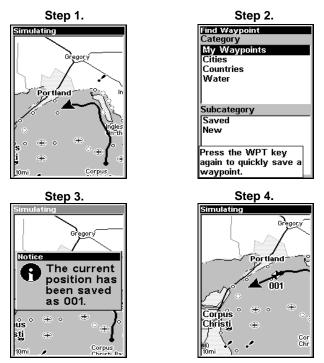
Sequence for setting a waypoint. Step 1: while traveling, *quickly* press WPT *twice* to call up Find Waypoint screen (seen in Step 2) and set a point. Step 3: a message says the waypoint has been saved. Step 4: vehicle continues on its way; number waypoint symbol is visible on map. NOTE:
